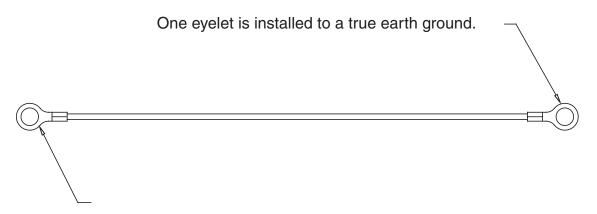
One eyelet is fastened to the pump hardware.
