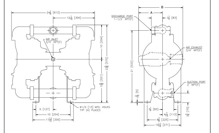
2" NPT(F) SUCTION • 1 1/2" NPT(F) DISCHARGE • 3/4" NPT(F) AIR INLET PORT • 3/4" NPT(M) AIR EXHAUST PORT
