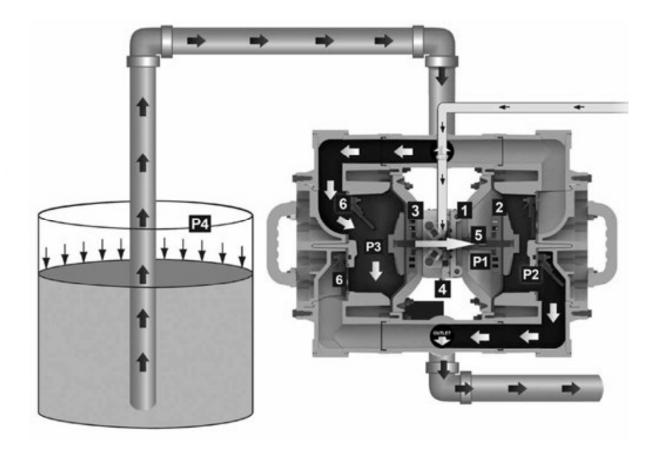
Air-Operated Double Disphragm (ACED) pumps are powered by compressed air or mirrogen.
