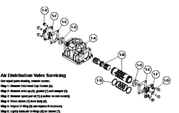
Rate: Seeve and speci (1) set almatch ground to a specified electronic steeve and specified (1) cannot be interchanged.
