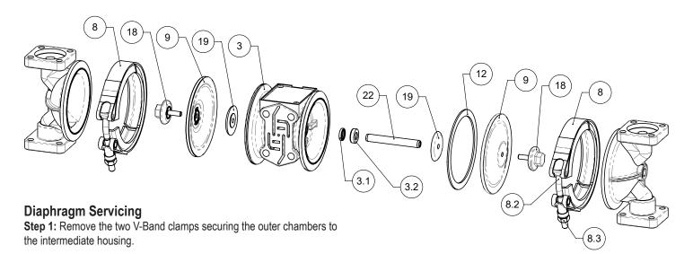
**Step 2:** Remove the diaphragm assembly (outer plate, diaphragm, spacer gasket (for PFTE units only, inner plate) by turning the assembly counterclockwise using a 1/2" (1.27 cm) wrench on the outer plate lugs. (If a socket is used, it must be a six-point socket.) The interior components consisting of the shaft seal and pilot valve assembly are now accessible for service.
