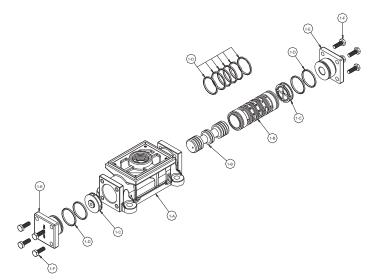
**Valve Assembly for Aluminum Mid Sections**
