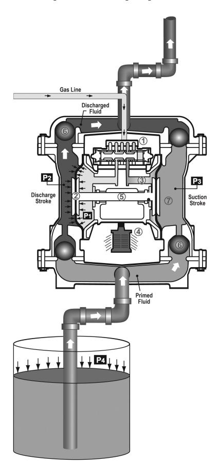
Gas-Operated Double Diaphragm pumps are powered by compressed gas, nitrogen or natural gas.
