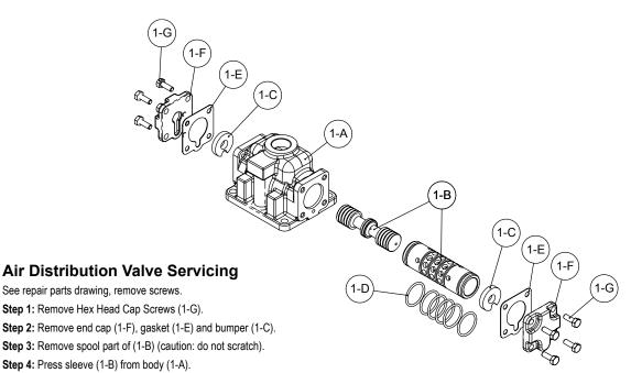
Step 5: Inspect O-Ring (1-D) and replace if necessary.
