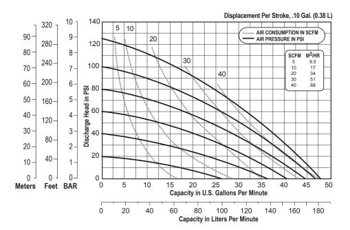
NOTE: Performance based on the following: elastomeric fitted pump, flooded suction, water at ambient conditions. The use of other materials and varying hydraulic conditions may result in deviations in excess of 5%.
