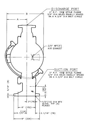
2" ASA STYLE FLANGED SUCTION AND DISCHARGE • %" NPT(F) AIR INLET PORT • %" NPT(F) AIR EXHAUST PORT
