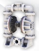
SOLIDS HANDLING Up to .71" (18 mm) MAX FLOW 238 GPM (901 LPM) MAX PRESSURE 100 psi (7 bar) DISPLACEMENT .9 gallon (3.41 liter)
