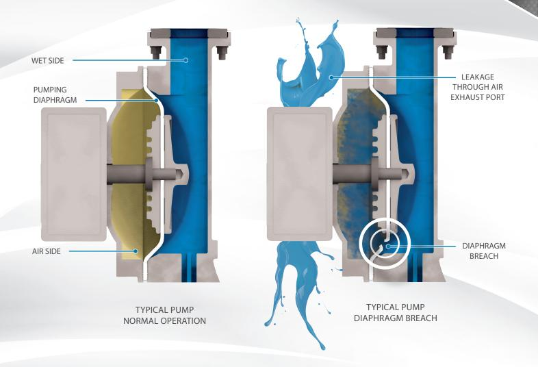
Typical AODD pump designs utilize a single pumping diaphragm to drive the fluid. The pumping diaphragm is the only barrier between the Wet Side and Air Side of the pump. This diaphragm is an elastomeric material that will eventually wear or become breached. When this occurs, the system fluid enters the Air Side of the pump and escapes to the environment through the air exhaust muffler. The pump must be immediately repaired or replaced.
