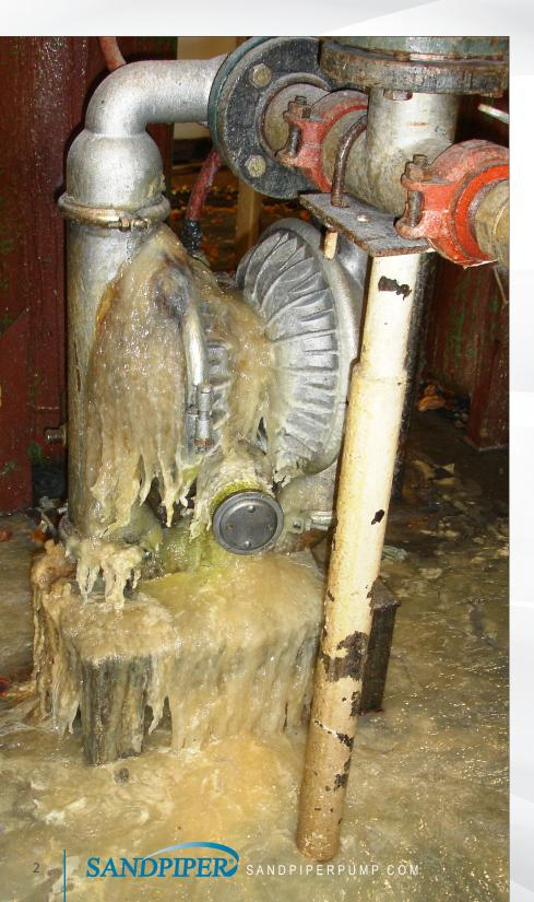
When the pumping diaphragm is breached, the fluid enters the air distribution system and escapes into the environment through the muffler, requiring immediate service. This results in:
