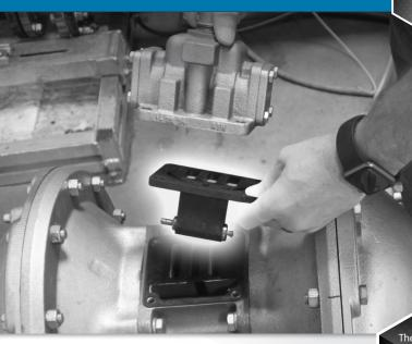
The Air Motor's Pilot Valve is the Most Often Serviced Part on an AODD Pump
