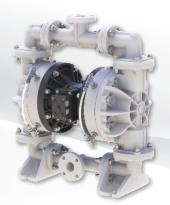
SOLIDS HANDLING Up to .47" (12 mm) MAX FLOW 100 GPM (379 LPM) MAX PRESSURE 100 psi (7 bar) DISPLACEMENT .43 gallon (1.63 liter)
