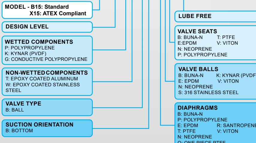
\*X Series ATEX pumps are ONLY applicable to Conductive Polypropylene pumps.
