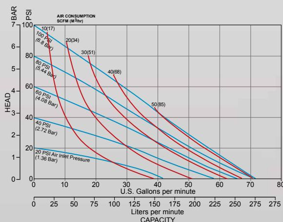
**Note:** The above Performance Curve has been determined under the following conditions: flooded suction, pumping clean water through a calibrated electronic flow meter with pulsation dampener and silencer fitted.
