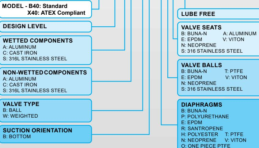
\*Pumps with cast iron wetted components are supplied at design level 01.
