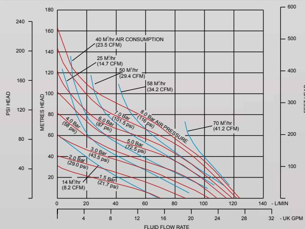
**Note:** The above Performance Curve has been determined under the following conditions: flooded suction, pumping clean water through a calibrated electronic flow meter with pulsation dampener and silencer fitted.
