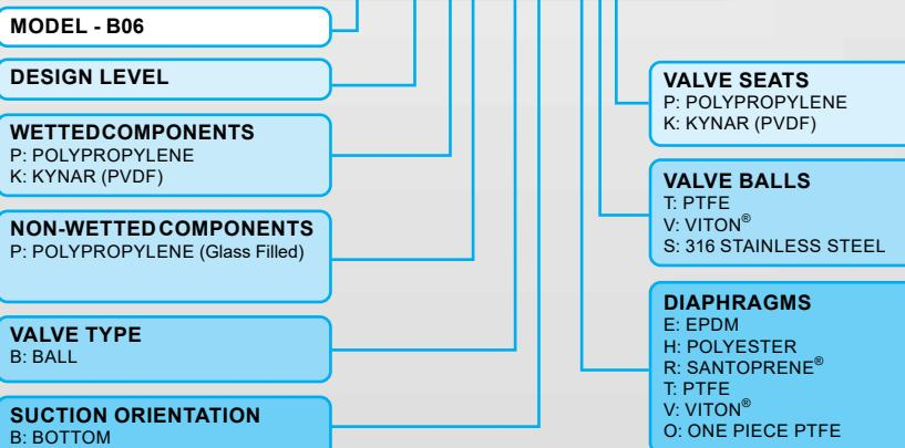
**Example above:** B06.04.PP.BB.TTP refers to B06 model, Design Level 4 with Polypropylene wetted components, Glass filled Polypropylene non-wetted components, with PTFE Diaphragms and Valve Balls and Polypropylene Seats.
