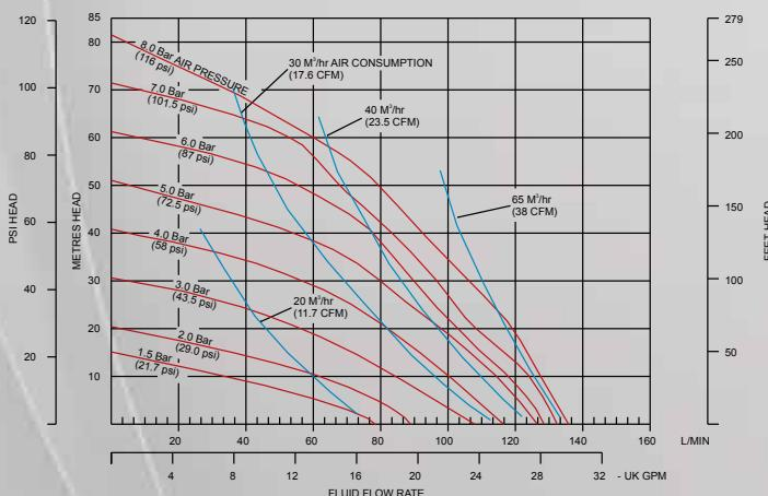
**Note:** The above Performance Curve has been determined under the following conditions: flooded suction, pumping clean water through a calibrated electronic flow meter with pulsation dampener and silencer fitted.
