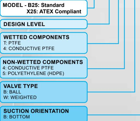
\*X Series ATEX pumps are ONLY applicable to Conductive PTFE pumps.
