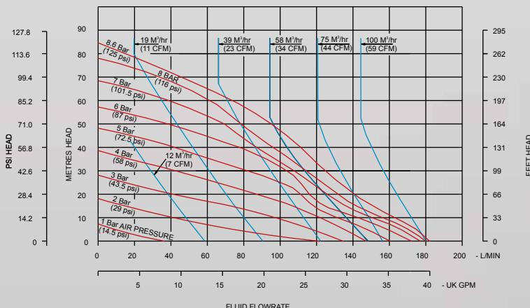
**Note:** The above Performance Curve has been determined under the following conditions: flooded suction, pumping clean water through a calibrated electronic flow meter with pulsation dampener and silencer fitted.
