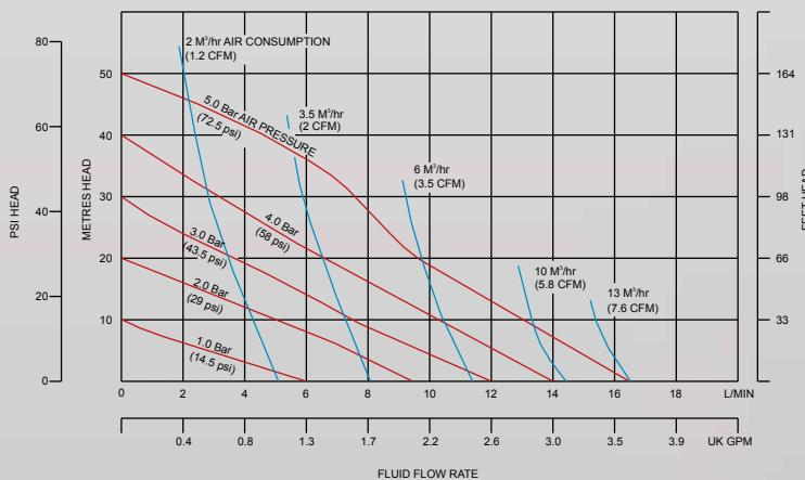
**Note:** The above Performance Curve has been determined under the following conditions: flooded suction, pumping clean water through a calibrated electronic flow meter with pulsation dampener and silencer fitted.
