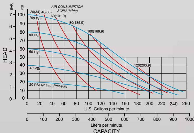
**Note:** The above Performance Curve has been determined under the following conditions: flooded suction, pumping clean water through a calibrated electronic flow meter with pulsation dampener and silencer fitted.
