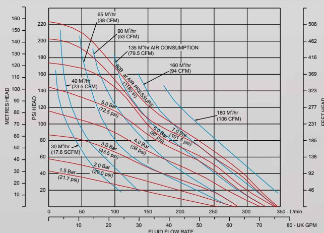
**Note:** The above Performance Curve has been determined under the following conditions: flooded suction, pumping clean water through a calibrated electronic flow meter with pulsation dampener and silencer fitted.
